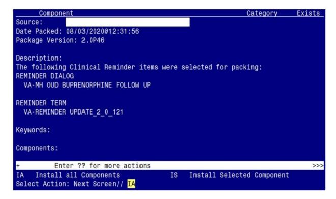
At the <u>Select Action</u> prompt, type <u>IA</u> for Install all Components and hit enter. Select Action: Next Screen// <u>IA</u> Install all Components
